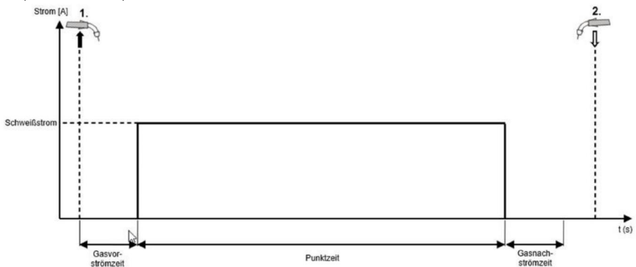
Fig. 7-5: Sequence of operation of the points mode
